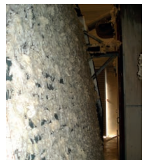
Inside the silo full of wool. The apron belt moves towards the silo.
