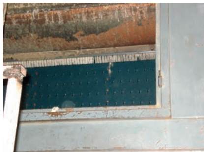
Expulsion roller at the top of the apron belt.
