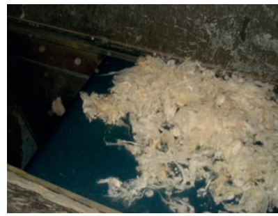
Belts that collect remains that fall from the expulsion roller at the back.
