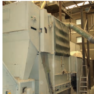
Loader at the back. The apron belt is at the front.
