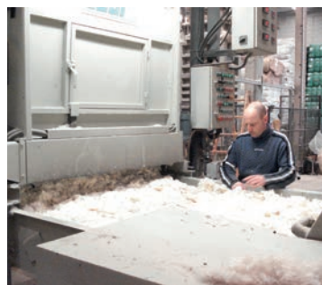
Manual separation of reject wool.
