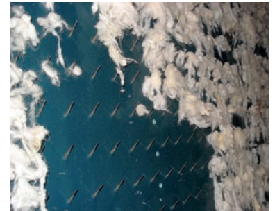
Detail of the apron belt that collects and opens the wool conveyed by the support belt.
