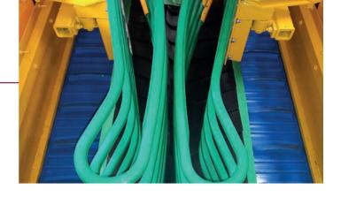
For optimum results mostgrape-harvesting machines choose to immobilise grapevines during the shaking process, avoiding risk of damage by friction between the grapevines and the grape-harvesting machine that take them directly to hoppers.
