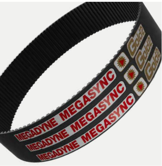
Gold2 belts have RPC profile, designed even to be interchangeable with existing deep toothed profile, which include HTB, RPP profiles and run on pulleys according to ISO 13050. MEGASYNC™ Gold2 belts are antistatic according to ISO 9563.
