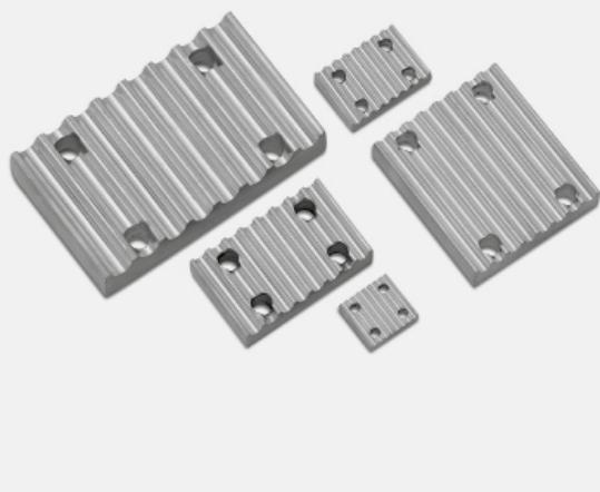
The clamping plates are used to fasten the ends of the open belts. On the customer's request, the plates can be delivered with or without fixing holes. As the belt can't be stretched with clamping plates installed we suggest to use other tension system. The plates are delivered in aluminium alloy.
