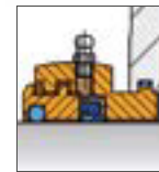
Taconite seal Multiple seal for harsh environments
