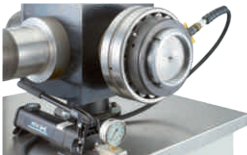
Extraction of the adapter sleeve with a hydraulic nut
