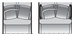
Fig. 19: The KIZEI® bearing is available in ISO widths, just like an open spherical roller bearing
