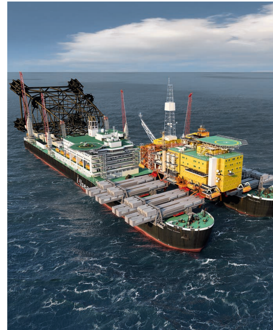
The world's largest special ship for the assembly and disassembly of oil drilling platforms
