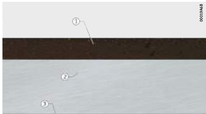
Figure 1 Maintenance-free plain bearing material E421
