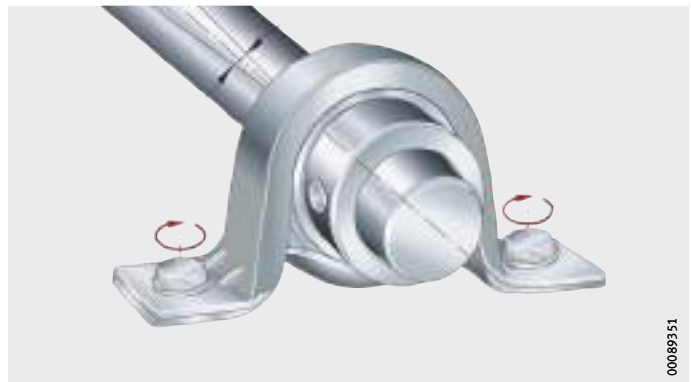
Figure 12 Screw mounting the housing finger tight
