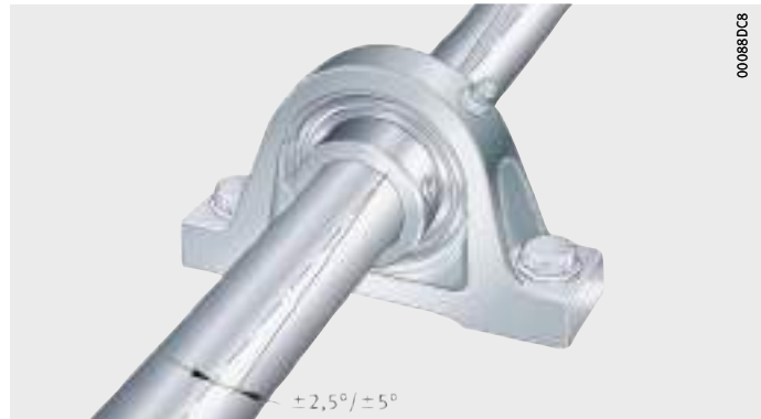
Figure 1 Compensation of static shaft misalignment
