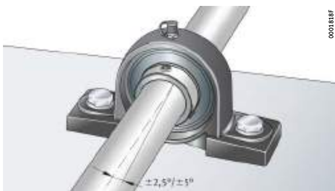
Figure 3 Compensation of static shaft misalignment
