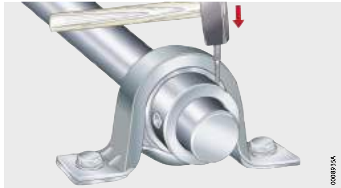
Figure 13 Tensioning the eccentric locking collar
