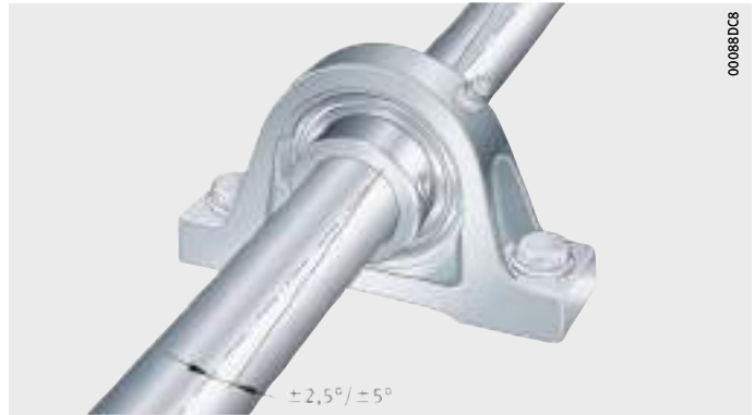
Figure 1 Compensation of static shaft misalignment
