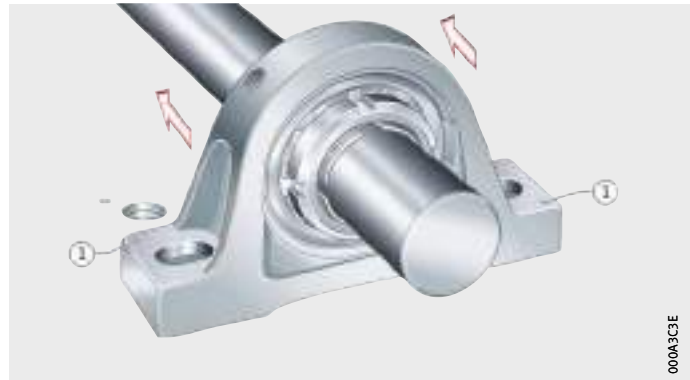
Figure 4 Sliding the unit onto the shaft
