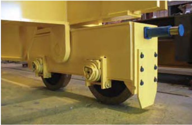
Fig. 5 Standard end cap design
