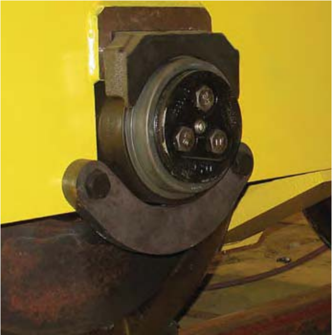
Fig. 8 Narrow adapter mounting on trolley safety bar
