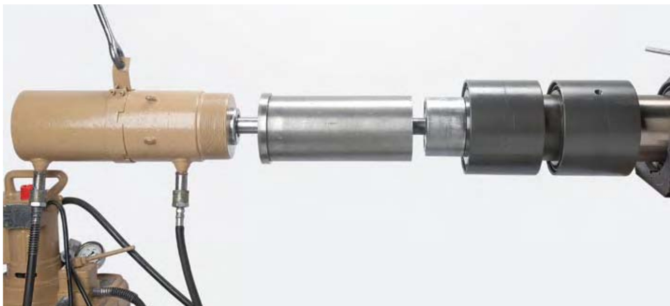
Fig. 28 Tooling used to push bearing onto shaft
