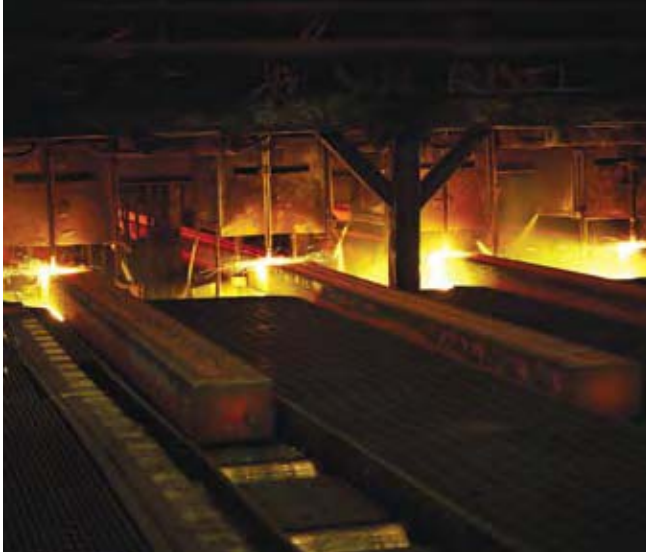
Fig. 11 AP bearing equipped runout tables
