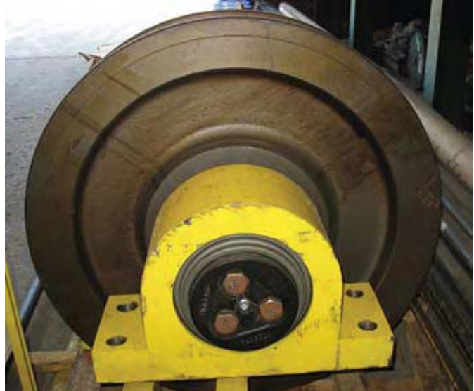
Fig. 12 AP bearings used in pillow block application
