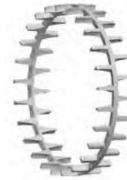
Fig. 45. One-piece, machined-brass, land-riding, finger-type cage.
