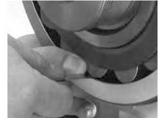
Fig. 92. During mounting, the RIC should be checked at the unloaded roller.
