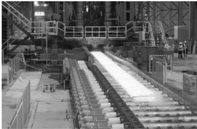
Fig. 113. Hot-strip mill transfer roller table.
