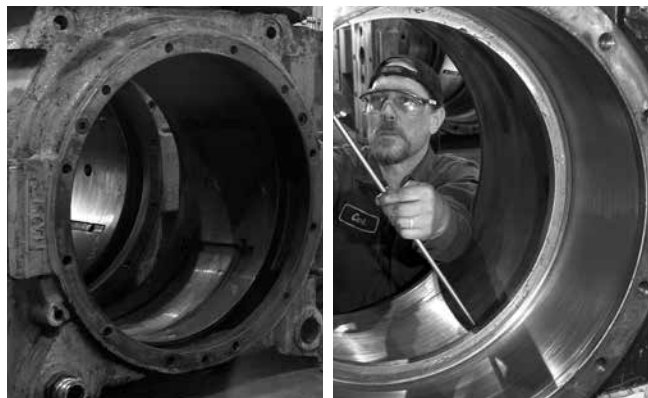
Fig. 278. Chock maintenance before and after photos.
