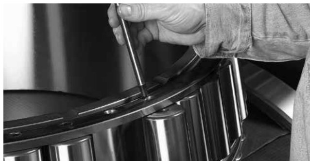
Fig. 232. Removing the threaded pin.
