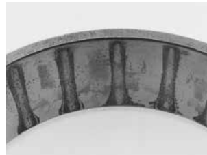
Fig. 189. Staining without pitting.
