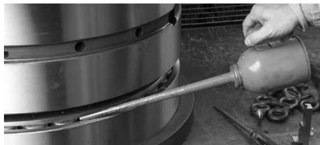
Fig. 267. Applying light oil to rollers and race.
