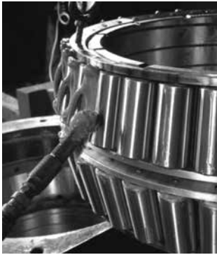
Fig. 245. Lubricating a tapered roller bearing with grease.
