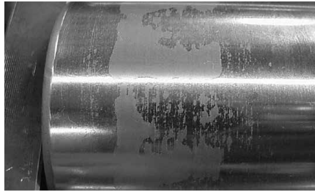
Fig. 184. Roller peeling damage.
