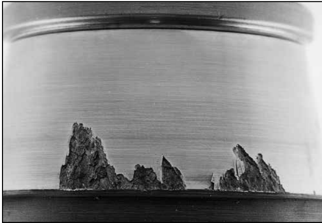
Fig. 171. Geometric stress concentration spalling.
