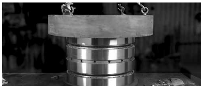
Fig. 265. Applied weight for seating rollers.
