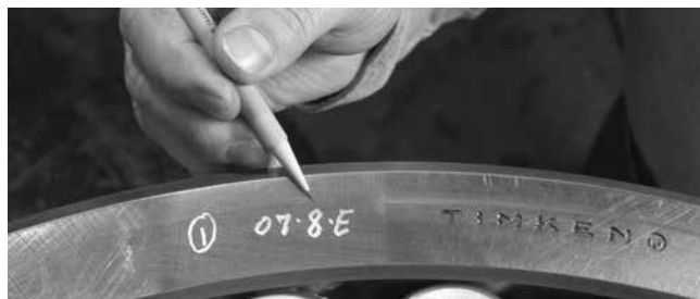
Fig. 266. Example of E cup marking.
