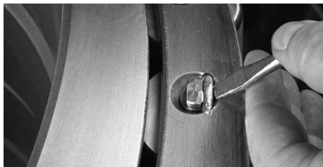
Fig. 231. Removing locking wire from an inspection pin.
