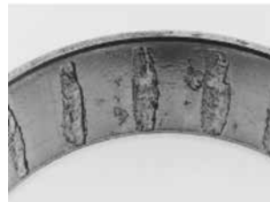
Fig. 191. Deep etching on an outer ring race.
