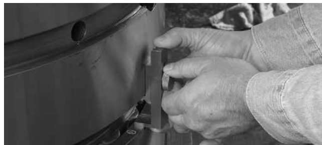
Fig. 268. Measuring B or D gap.
