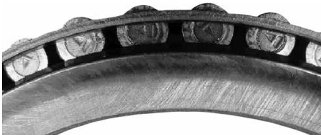
Fig. 183. Roller end and rib discoloration.
