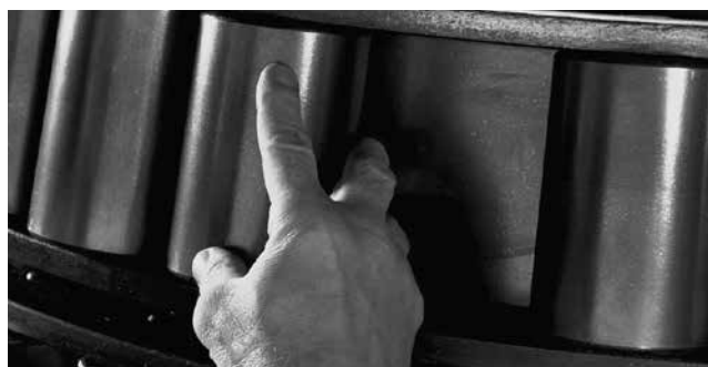
Fig. 233. Inspecting inner race.
