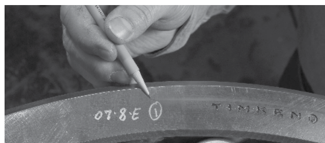
Fig. 226. Example of quadrant marking.
