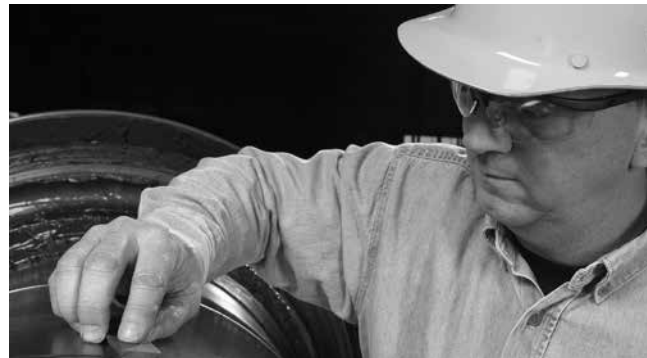
Fig. 240. Restoring minor roll neck damage.
