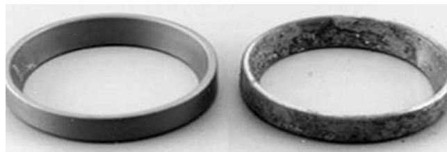
AquaSpexx® cup after testing Uncoated cup after testing
