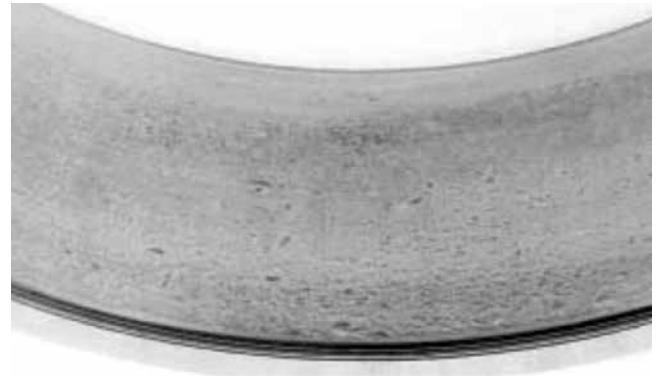
Fig. 160. Bearing damage due to abrasive particles.
