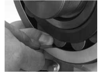
Fig. D-4. During mounting, the RIC should be checked at the unloaded roller.
