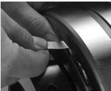
Fig. D-7. Measure RIC before installation.
