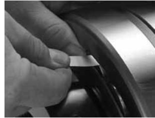
Fig. D-3. Measure RIC before installation.
