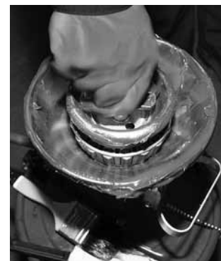
Fig. 22. Mechanical grease packer.
