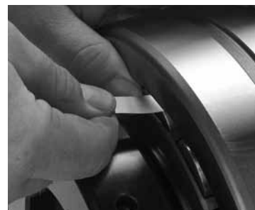
Fig. 18. Measure RIC before installation.
