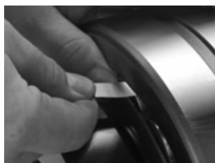
Fig. 14. Measure RIC before installation.
