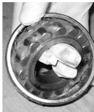
Fig. 21. Grease can easily be packed by hand.
