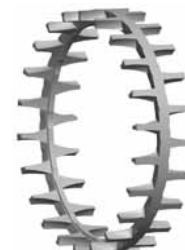
Fig. 6. EMB/YMB One-piece, machined-brass, land-riding, finger-type cage.
